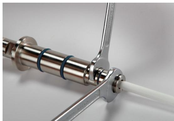
Figure 8: Tighten the cap nut
