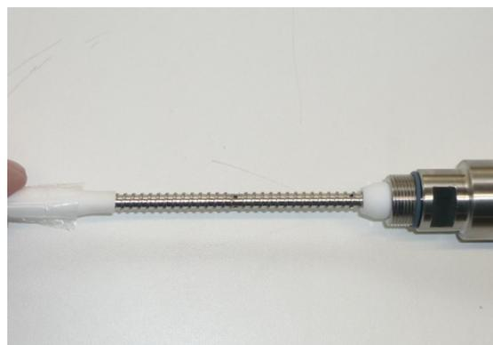
Figure 6: Mount the polypropylene membrane
