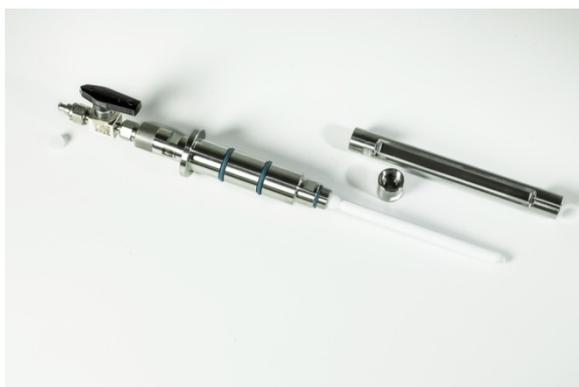
Figure 7: Mounted polypropylene membrane
