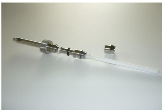
Figure 9: Mounted polypropylene membrane
