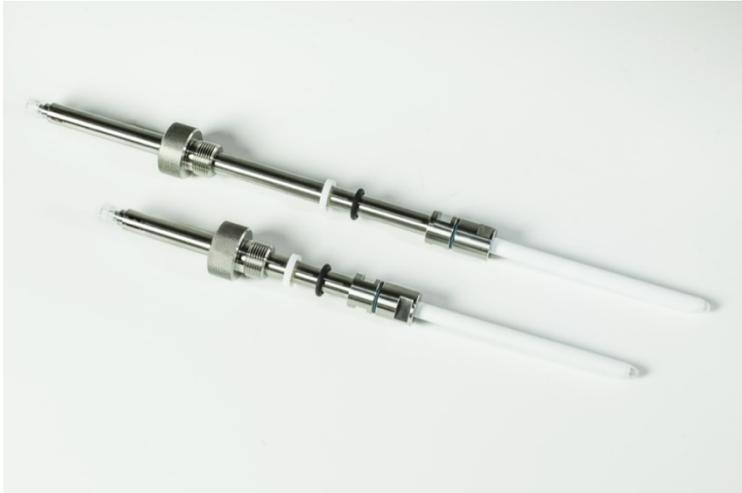
The filtration probe is sterilized together with the bioreactor and installed in a 12 mm top port with PG 13.5 thread or in a 19 mm top port using a 19/12 mm reducing adapter.
