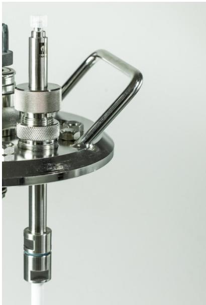
After installation, please ensure that the probe does not come into contact with moving parts (e.g. stirrer or agitator shaft) inside the bioreactor.
