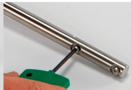
Figure 13: Tightening the 2 screws
