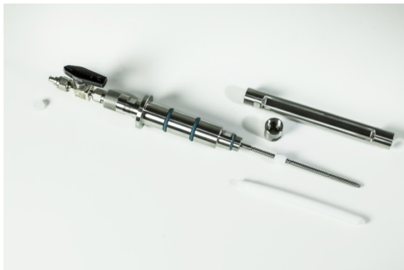
Figure 3 and 4: Insertion of the PTFE ferrule
