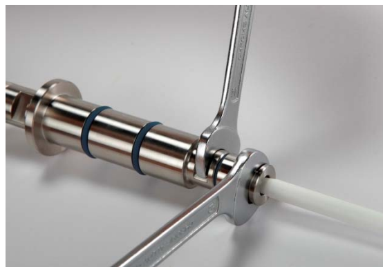
Figure 7: Tighten the cap nut
