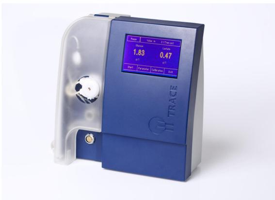
The detection is performed using a combination of an enzymatic reaction with an amperometric detection. Glucose is converted via glucose oxidase to gluconolactone and hydrogen peroxide. This is measured at a platinum electrode. The biosensors have life time of 5000 measurements or 21 days.
