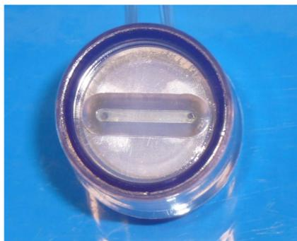
The membrane acts as a sterile barrier and is used for the separation of the analytes of interest. The dialysis plug is installed at the bottom side and sterilized together with the disposable bag.
